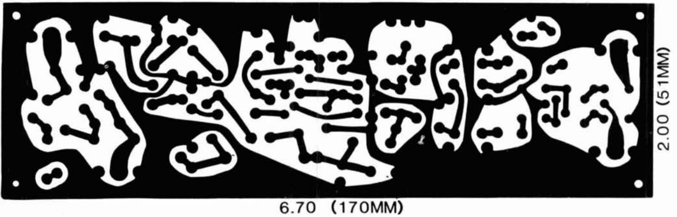
Transmitter board PC layout.
